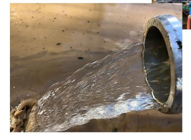
Discharge to be stored as recycled water and reused. NTU Is down to <u>7</u> From over 1000 NTU
